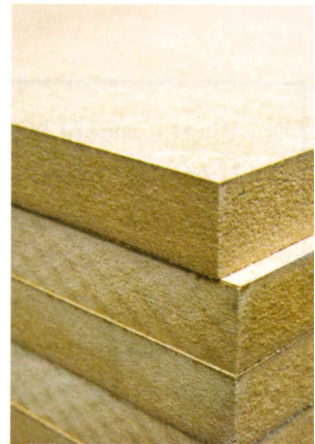
MDF – medium density fibreboard
