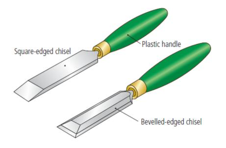
The bevelled edges allow the chisel to fit into tight corners such as a dovetail
