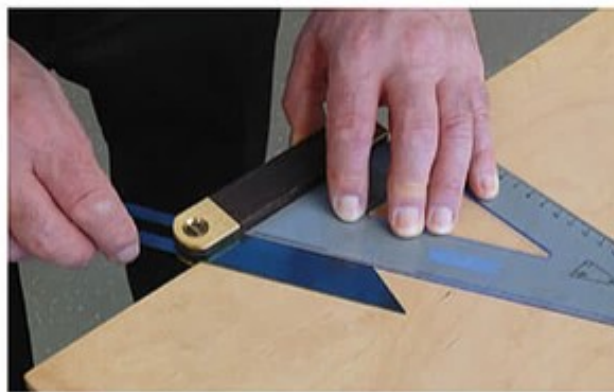
Sliding bevel being set to a setsquare
