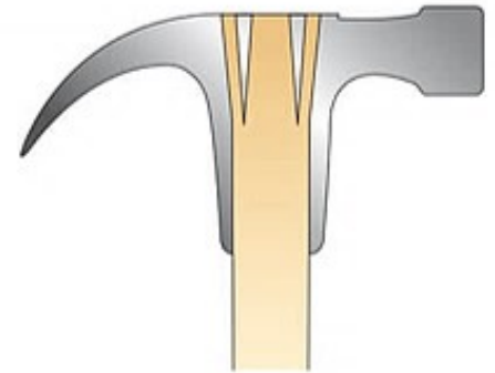
The head of a hammer is held on with wedges
