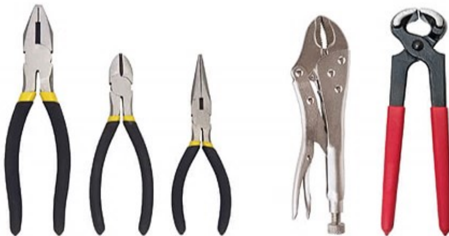
Combination pliers, wire cutters, long nose pliers, vice grips, pincers (left to right)
