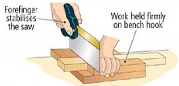
Using the tenon saw
